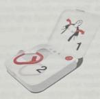
7 Pull the red handle to reveal the electrode pads.
